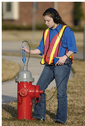
Leak Detection Technician "sounding" at a fire hydrant to verify leak
