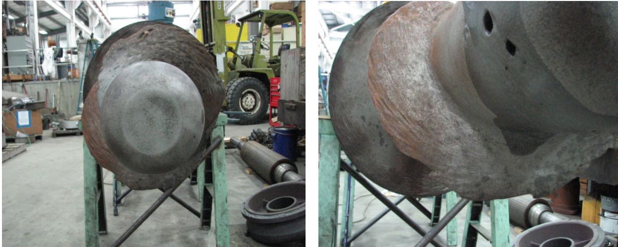
Mixer assembly after sandblasting, showing substantial impeller wear and pitting
